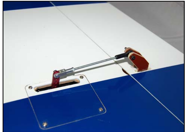
(above) Aileron linkages are assembled using the provided hardware. Outer servo hatch is secured with Ø 2.9 x 10mm screws. Mill the slots in the hatches to suit your metal servo arms.
