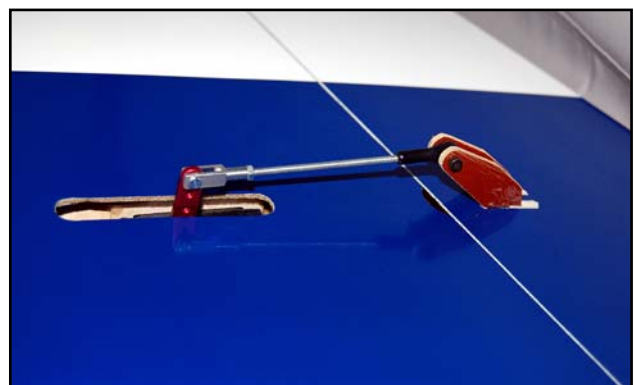
(below) You must use full metal servo arms, like the 1.5" SWB arms shown here.
