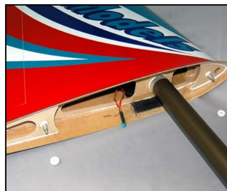
(below) The wing root, showing the 50mm Ø 6061 alloy wing tube and the aluminium anti-rotation dowels.
