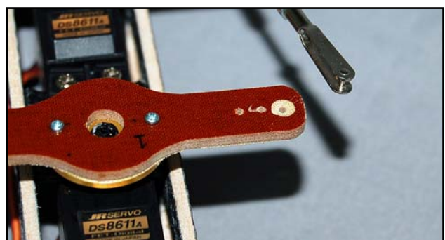
(below) Sand small rounded dimples about 0.5mm deep for proper clearance of the M3 steel clevises, only on one side of each phenolic horn, as shown here.
