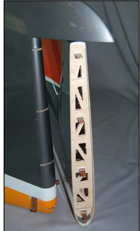
(above) The lightweight fin-post has the phenolic rudder hinge posts already installed and aligned at the factory. The corresponding tubes are also installed in the rudder for the hinge tube.
