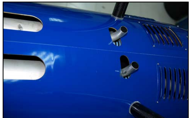
(above) Make two small 40 x 25mm wide slots for the muffler exits.
