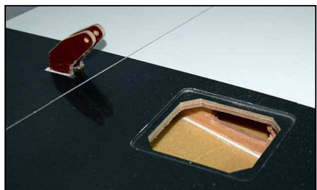
(below) Access to the outer servo is through the milled servo hatch provided. Glue the supplied plywood doubler to the inner face of the rib and secure the servos with Ø 2.9 x 16mm sheet-metal screws.
