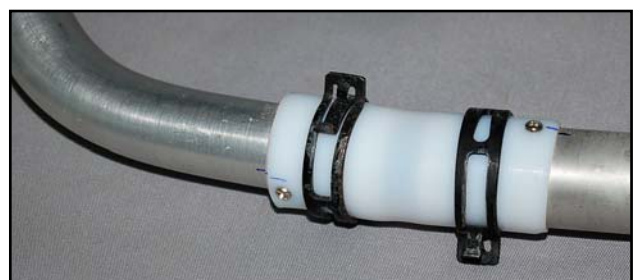
(below) 2 small screws thru' the Teflon joiners prevent the cans moving in flight.
