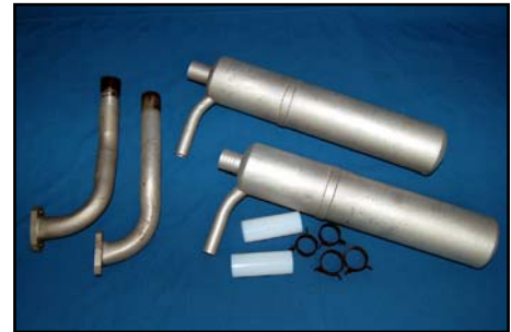
(above) MTW headers & canisters are available as optional items from C-ARF. Shown here are the TD110 cans and headers for the DA-150. (below) Support bulkhead securely glued into position in the muffler compartment with epoxy and micro-balloon mixture.
