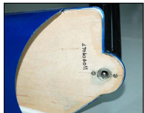
(left/below) Completed wheelpant with 5" Dubro wheels. The angle of the wheelpants to the legs is set with 2 small sheetmetal screws, thru' the wheelpant into the carbon leg.
