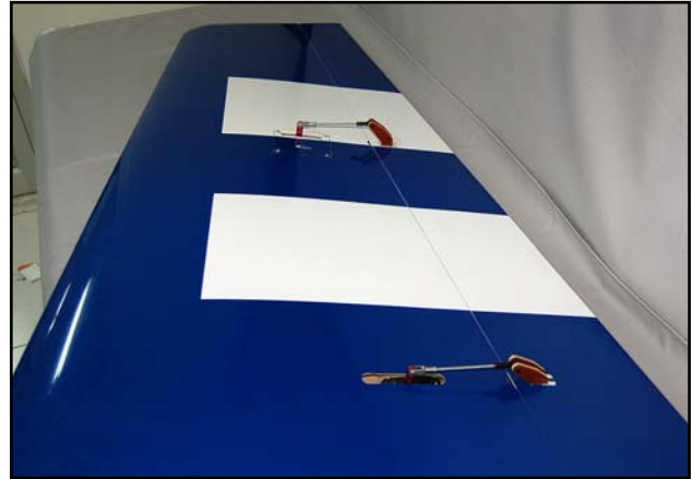
(above) Each aileron is controlled by two JR 8511/8611 servos, or stronger, that fit into milled cutouts in the ribs.
