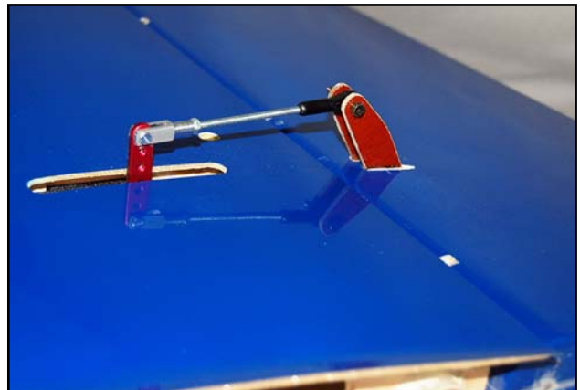
(below) Milled 3mm thick plywood doublers are included for both the JR8711/8811 and the Futaba S9152 servos. JR8811 and SWB 1.5" servo arm shown here.
