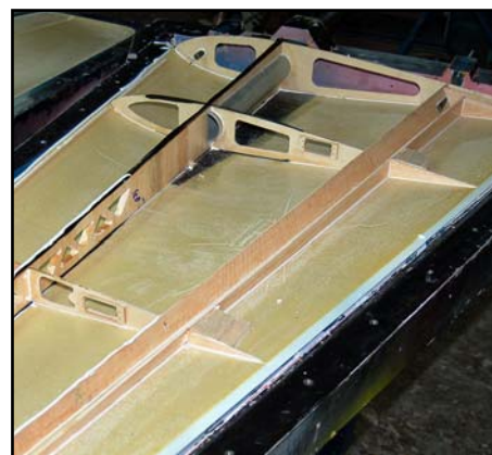
(above) The internal wing structure, showing the 3mm plywood doublers on the outside of both milled servo mounts.
