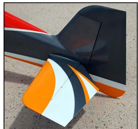
(below) The elevator and rudder hinging uses 4mm diameter tubes, inside phenolic hinge posts that are factory-installed and aligned.
