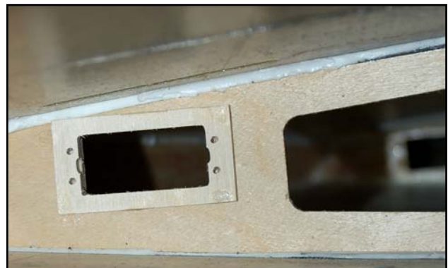
(below) Access to the outer servo is through the milled servo hatch provided. Glue the supplied plywood doubler to the inner face of the rib and secure the servos with Ø 2.9 x 16mm sheet-metal screws.
