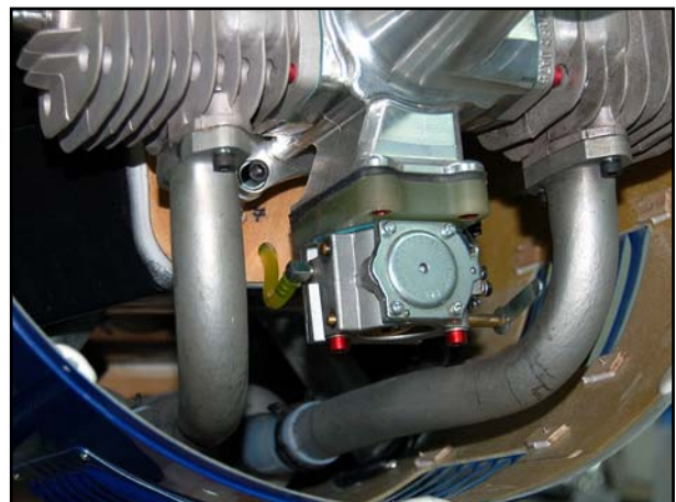
(below) Another DA-150 view showing the headers and the location of the hole thru' the firewall for the Tygon fuel tube.
