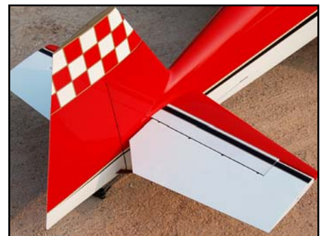
(below) The elevator hinging uses 4mm diameter aluminum tubes, inside phenolic hinge posts that are factory-installed and aligned.
