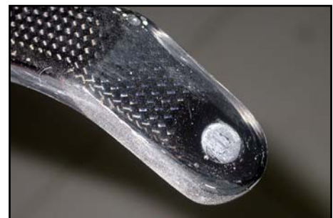
(above) The moulded dimple in the bottom of the carbon legs. Drill a central hole of 6mm diameter.
