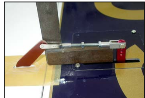
(above) Clevis hole for inboard horns should be 23 - 24mm from aileron surface, and perpendicular to the aileron front edge.
