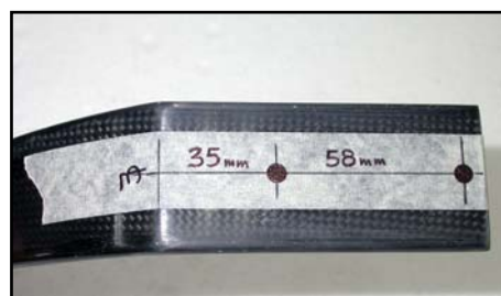
(below) Drill 2 x 6.5mm Ø holes for bolting in the Landing Gear.
