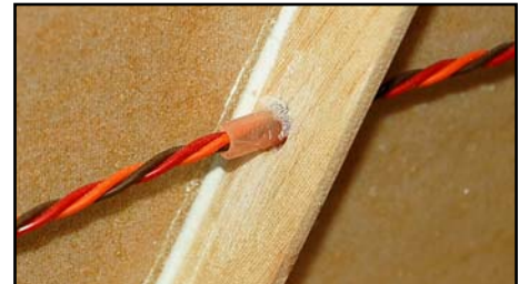
(above) Protect all wires and tubes where they pass thru' bulkheads, or near sharp composite parts, with a short length of silicone tube, and fix firmly in position.
