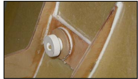
(above) Plywood rings glued in vertically for front nuts with thick mixture of epoxy/micro-balloons.
