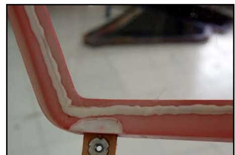
(below) When fixed, remove frame & secure edges of canopy firmly with epoxy/micro-balloon mixture
