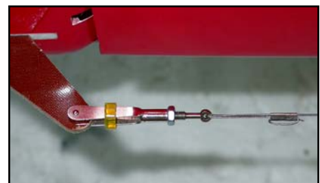
(below) Pass rudder cable thru' crimping tubes 2 times for safety, and prevent all clevises from opening with small pieces of tubing.
