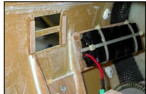
(below) Powerbox, Receiver and switch location in the Extra 300SX.
