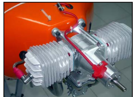
(below) DA-100 mounted on a 330L. The mounting system is identical for the 300SX, except that you will need 30mm long stand-offs, and accurate thrustline alignment is even easier!
