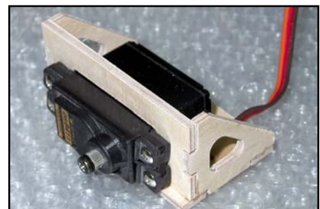
(above) Throttle servo mount assembled from milled plywood.
