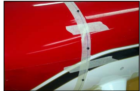
(above) Cowling is secured with nine M3 bolts, into T-nuts fitted in reverse, glued inside fuselage with a thick micro-balloons mixture.
