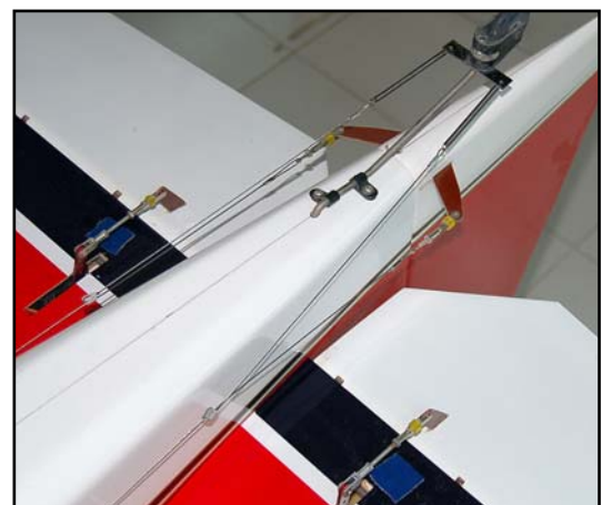
(below) Tailwheel assembly can be connected to rudder horn OR rudder cables with springs for improved steering.
