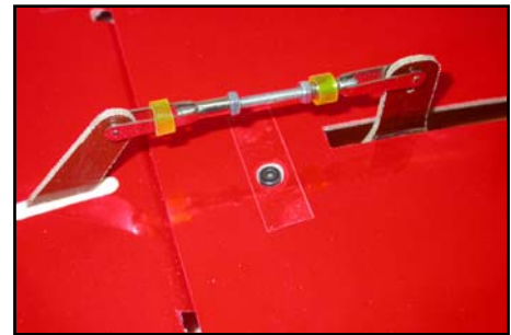
(above) Shows the stab retaining bolt, with clear tape over it to prevent it coming out in flight. The small pieces of tubing stop the quick-links from opening.
