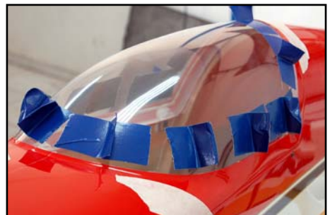
(above) Use duct-tape handles to pull the clear canopy tightly against the canopy frame while gluing it in position with a few very small drops of odorless-CA.
