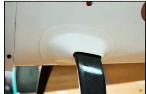
(above) Fibreglass leg Cuffs are secured to fuselage with a little clear silicone adhesive, allowing easy removal if necessary.
