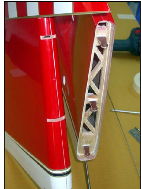
(above) The lightweight fin-post has the phenolic rudder hinge posts already installed and aligned at the factory. The corresponding tubes are also installed in the rudder for the hinge wire.
