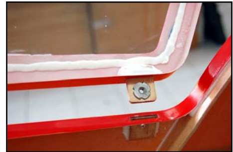
(above) The canopy frame is secured to the fuselage with 4 tabs, M4 bolts and T-nuts, all finished at the factory for you.
