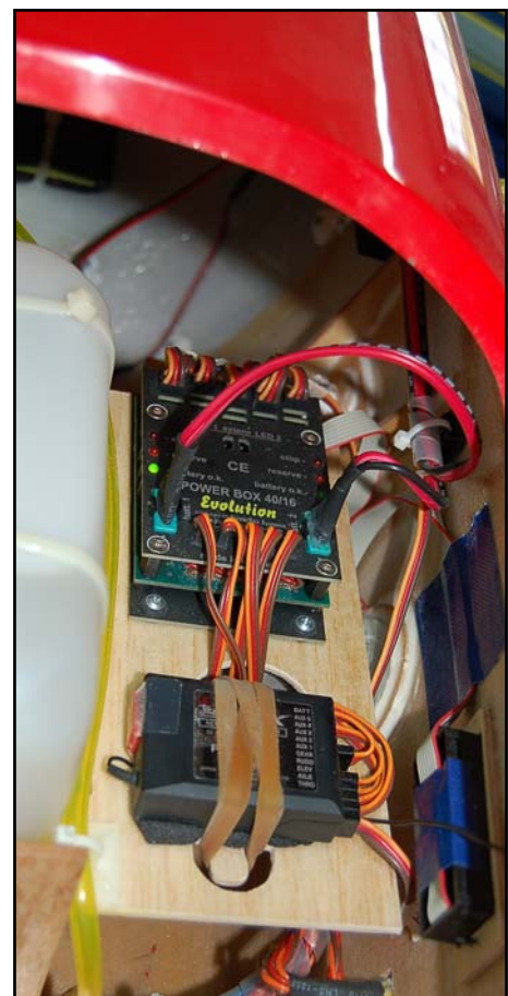
(below) Powerbox, Receiver and switch location in the Extra 300SX.
