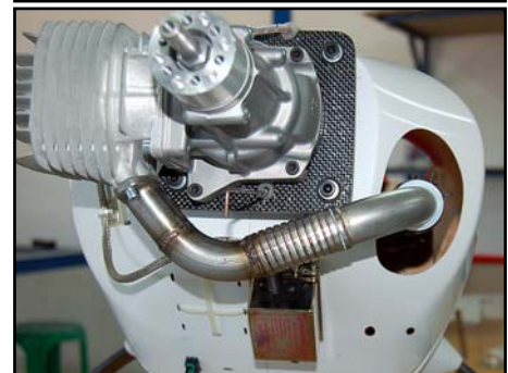
(above) 3W 80cc Xi motor installed, with custom header and Greve tuned pipe. Note position of Ignition unit, and cable -ties which secure the 2 receiver Nicads inside the motordome.
