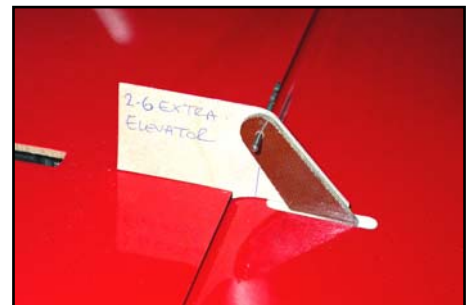
(below) Elevator horn alignment template from scrap plywood. Line is hinge axis. Use for both elevators to ensure same throws.
