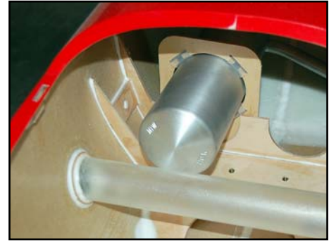
(above) A single 80mm Ø can (TD110K shown) can be fitted - but you may need to use a cross-over header to get the correct length.
