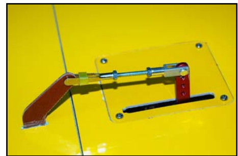
(above) Outer aileron horn. Clevis hole is 30mm from aileron surface.
