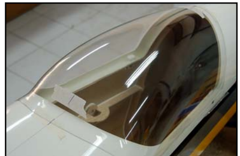
(above) Mark centrelines on the clear canopy at front and back and visually check that it is straight. (below) Duct-tape handles used to pull clear canopy against the canopy frame while gluing it in position with a few small drops of odorless-CA. Remove canopy and secure the edges of the clear canopy with a bead of epoxy to trap it in place (see above)
