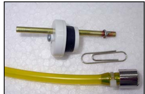
(below) Secure the connectors between the motor & ignition unit. (below) Fit barbs to all brass tubes and fuel connections for safety. Easily made from a paper-clip, soldered onto the brass tubes.
