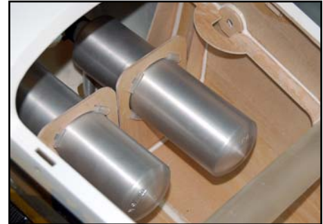
(above) Plenty of room to install a pair of MTW 75K cans in front of the wing tube, supported with the milled mounts supplied in the kit. (below) Typical cnc milled plywood canister/tuned pipe mount & hard silicone tubing included in the kit to suit Ø 49mm pipes, and both Ø 70mm & 80mm canisters.
