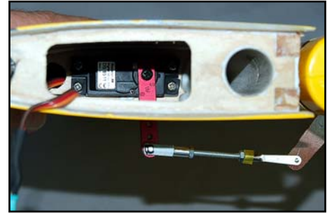
(above) Servo is screwed into the milled cutout in the inner rib.
