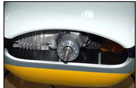
(above/below) Baffle installed in the cowl for the 3W motor.
