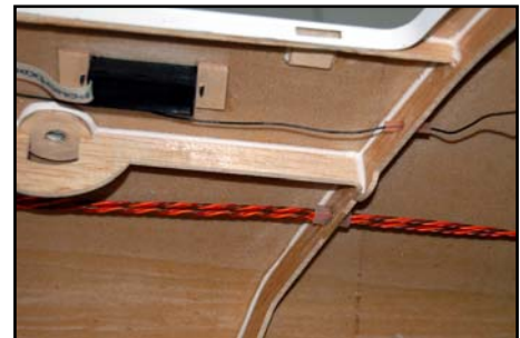
(above) PB Switch mounted in fuselage side, with ply reinforcement. Antenna wire and stab extension cables are routed thru' silicone protection sleeves and fixed securely.
