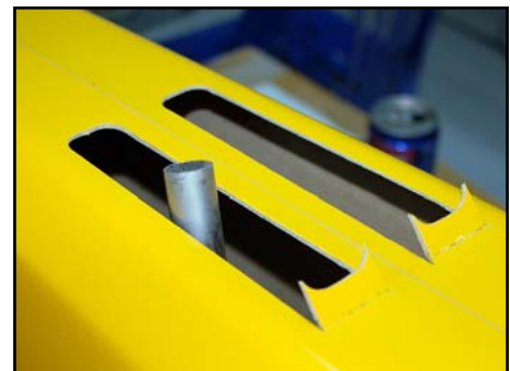
(below) Radius the corners of all air exits, and cut angled tabs at the front to create some turbulence & make sure the air is sucked out.
