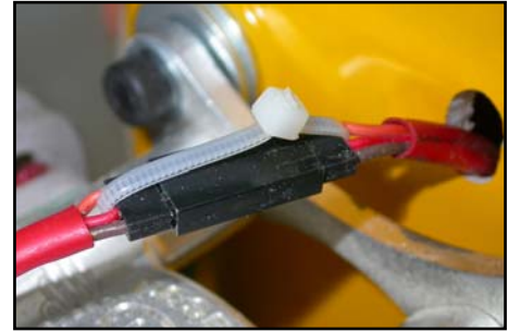
(below) Secure the connectors between the motor & ignition unit. (below) Fit barbs to all brass tubes and fuel connections for safety. Easily made from a paper-clip, soldered onto the brass tubes.
