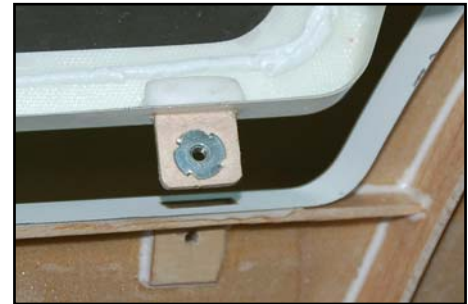
(above) The canopy frame is secured to the fuselage with 4 tabs, M4 bolts and T-nuts, all finished at the factory for you. Also note the bead of epoxy to secure the canopy to the inside of the fibreglass frame.
