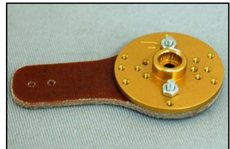
(above) If you use the phenolic servo arm extensions, you MUST bolt these to metal servo discs.
