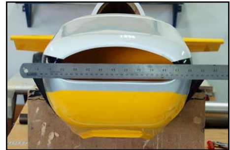
(above) Check cowl opening is parallel to stab or wing tube, and tape in position.
