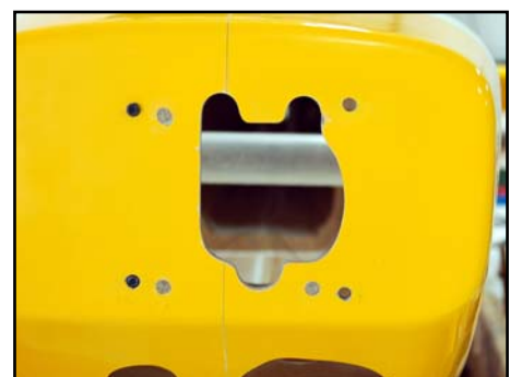
(above) Shows the cutout for the 3W carb, and also the holes from the DA-100 mount plugged with 6mm hardwood dowels.
