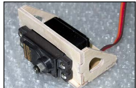
(above) Throttle servo mount assembled from milled plywood. (below) In the 3W set-up this was glued to the top of the fuselage
