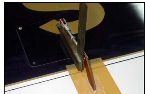
(below) Make sure control horns are perpendicular to aileron surface and parallel to servo arm.
