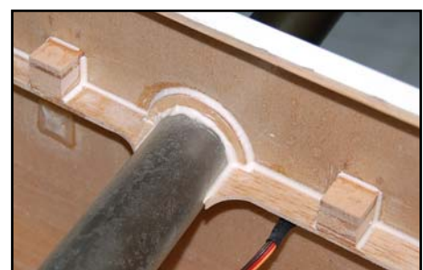
(bottom) Tank base is fixed to the blocks with 4 of the large sheet-metal screws, and washers.
