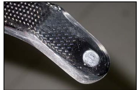
(above) The moulded dimple in the bottom of the carbon legs. Drill a central hole of 6mm diameter. (below) shows the M3 bolt thru' the carbon leg, into the T-nut glued inside the wheelpant.
