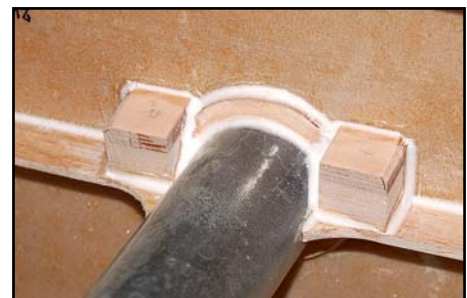
(above/below) Make 4 blocks from the balsa & plywood parts - and glue securely into position.
