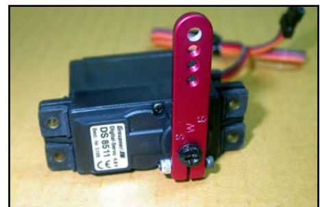
(below) The alternative is full metal servo arms, such as these SWB 'Double-Loc' types that we use on most of our factory planes.
