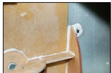
(above & below) Tack glue the T-nuts in position with a small drop of thick CA first. When cowling is correct, secure all the T-nuts with a drop of, fairly wet, epoxy and microballoons mixture as shown.
