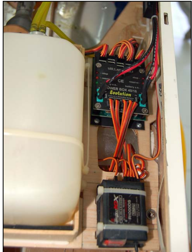
(above) There is plenty of space to fit the Powerbox Evolution and Rx on the right (or left) side of the fuel tank base.
