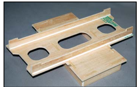
(above) Tank base assembled. Production base is larger giving space for receiver and Powerbox.
