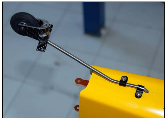
(below) Tailwheel assembly installed. It can be connected to rudder horn OR rudder cables with springs for improved steering.
