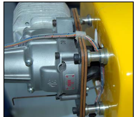
(below) Sidethrust and upthrust are set with stacks of large diameter washers between the 20mm standoffs and firewall. The wire below operates the choke.
