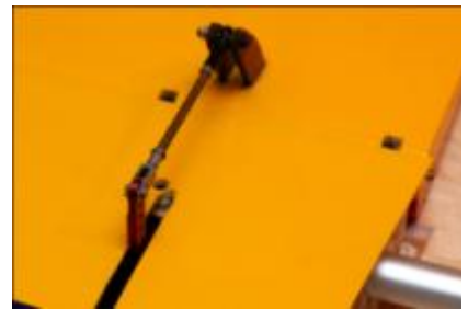
Linkage with a ball-link on the control horns and a clevis in the aluminium servo arm.
