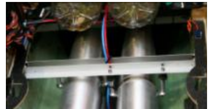
The tuned pipes installed at the fuselage
