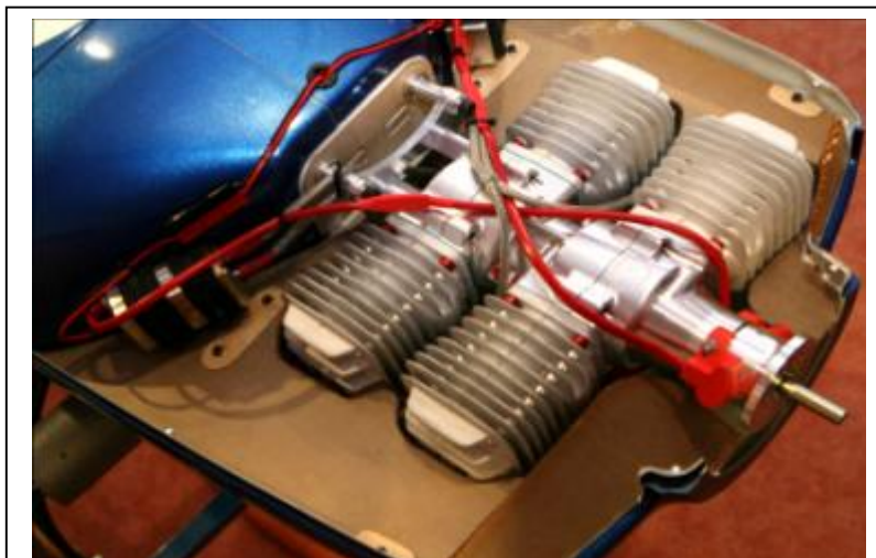
It's important that the baffle plate for DA200 encloses the whole engine as you can see above. It consists of three parts which are fitted by M3 screws.
