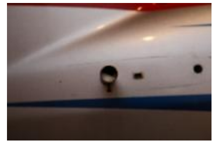
Rear stab spar tube has M3 T-nuts installed at the factory for the securing bolts.
