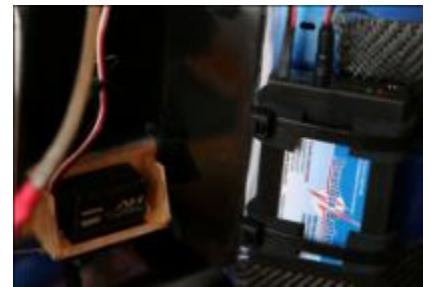
The ignition battery and the throttle servo installed at the dome (DA170)
