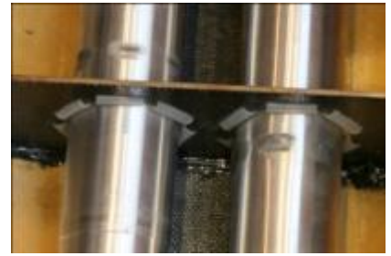
That may happen to your canisters, if you don't reinforce the bearing position
