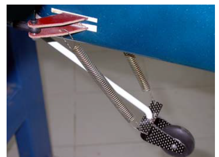
Connect the steering arm to the rudder horns with springs for steering option if required.
