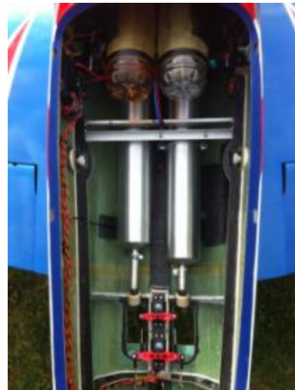
Position of the rudder tray when installing DA170 on tuned pipes
