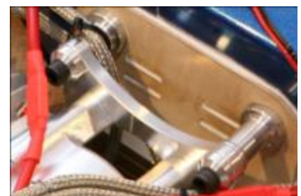
CNC milled distances. Alternatively you can use a pack of washers. Top right 18mm Top left 24mm Bottom right 21mm Bottom left 27mm
