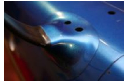
The leg cuffs glued in place onto the LG with silicone.
