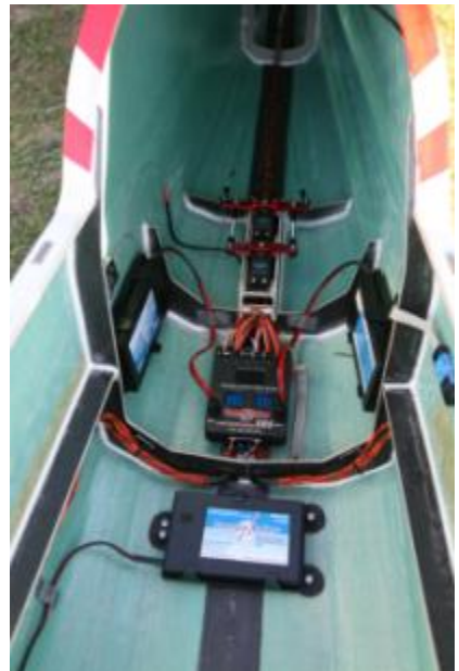
RC-installation for DA200. If you intend to fly more pattern, you can install the ignition battery a bit closer to the front.
