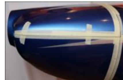
The cowl firmly taped in position
