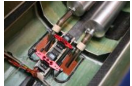
The exhausts made of VA tubes and the reinforced cutouts
