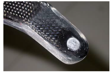
The moulded dimple in the bottom of the carbon legs. Drill a central hole of 6mm diameter.
