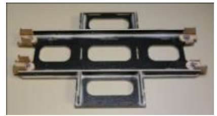
The fuel tank base prepared for PET-tanks together with the four mounts
