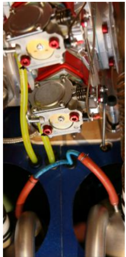
The rubber grommets to protect the tubes
