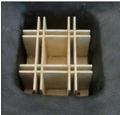
The plywood cuboid together with the carbon fibre extension
