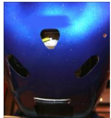
The cutouts in the cowling (DA170 on tuned pipes)
