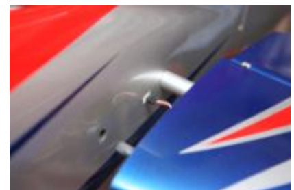
A plug at the fuselage connects the elevator servos to the RC-System
