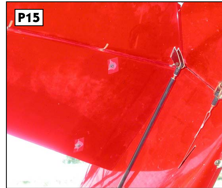
P15 General view of elevator and rudder linkages, also shows stab retaining bolts and clear tape.
