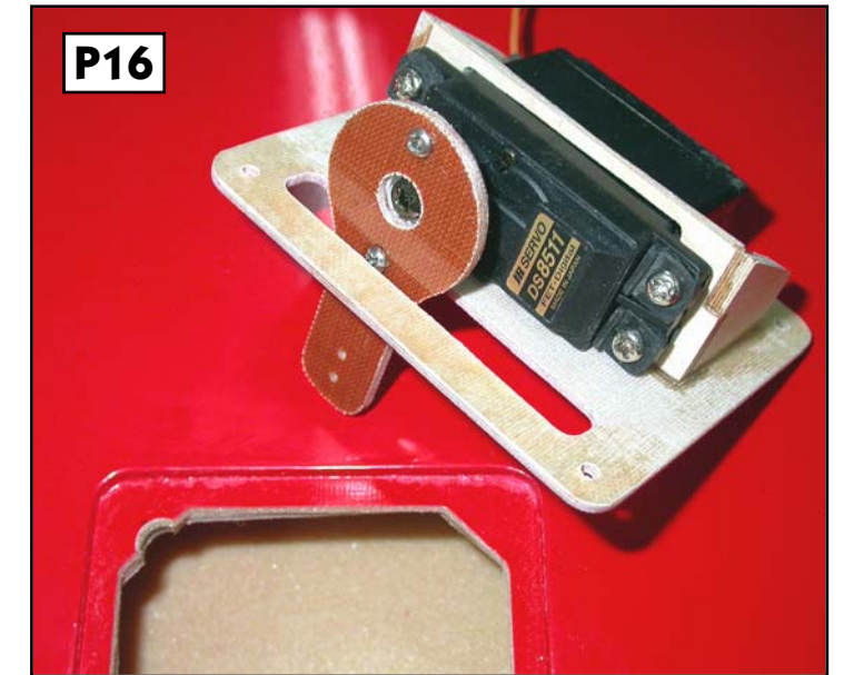
P16 Typical aileron mounting from cnc milled ply parts. Make sure you secure with a fillet of epoxy all round the joints.
