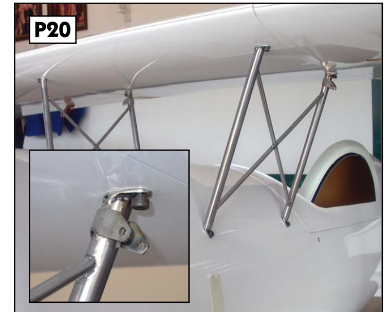
P20 General view of stainless steel cabane struts and connection with M4 bolt into blind nuts.
