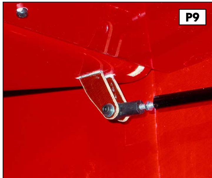
Tape handles to aid gluing clear canopy into frame. (below) Elevator linkage details (brass tube not shown)
