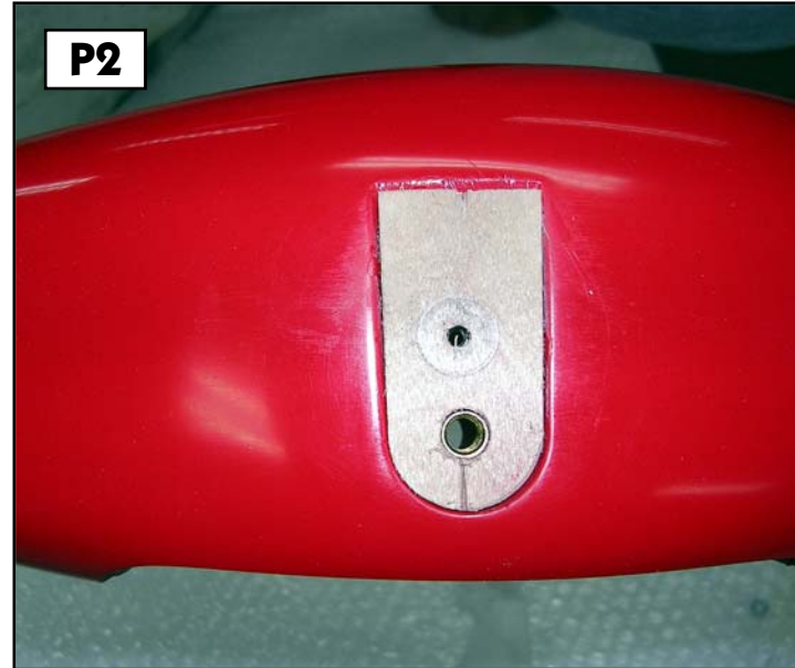
Milled plywood plate glued to wheelpants.
