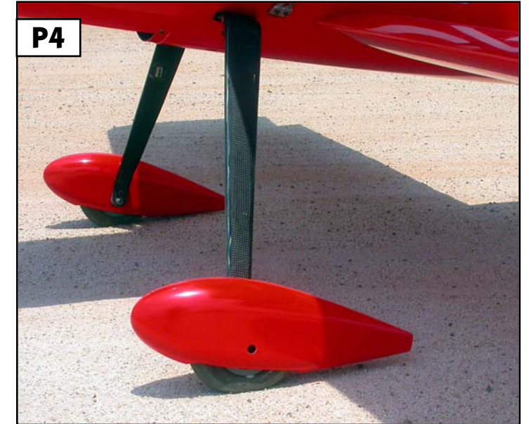
Wheelpant angle set so that back end just clears the ground.
