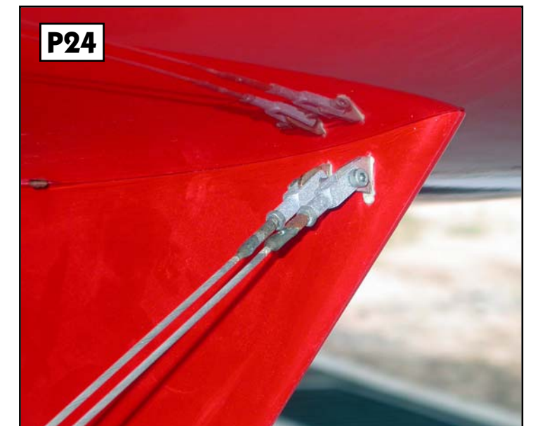
P20 General view of stainless steel cabane struts and connection with M4 bolt into blind nuts.
