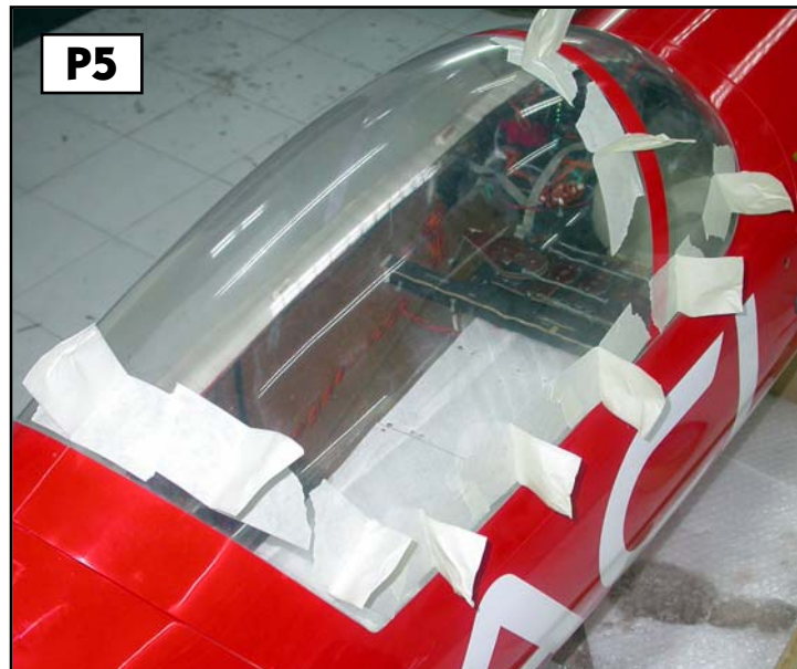
Tape handles to aid gluing clear canopy into frame. (below) Elevator linkage details (brass tube not shown)
