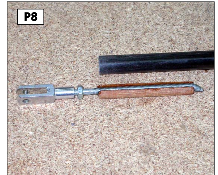
M3 threaded rod in wood dowel glued into carbon pushrods. (below) Cable separator and pushrod supports.
