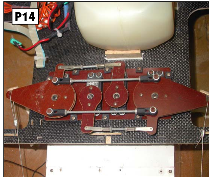
P14 Completed rudder servo linkages. Note phenolic arms also secured with minimum 2 sheetmetal screws each.
