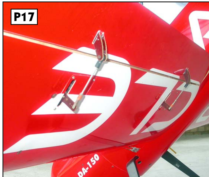
P17 Aileron linkages on bottom left wing. (below) Aluminium inserts in outer struts fit into moulded pockets in wings.
