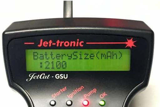
The battery capacity is used to calculate the charging level/remaining energy of the engine supply battery.
