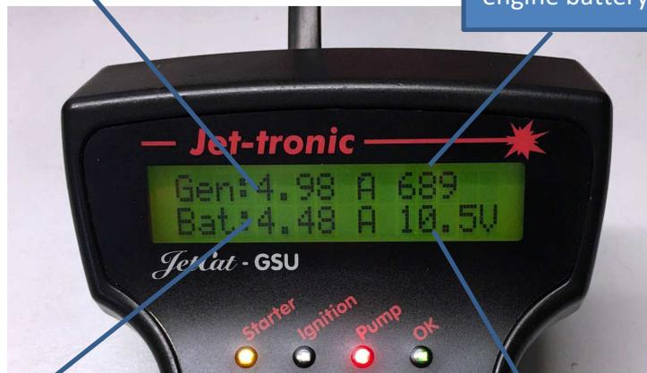
Charging current into or out of the engine battery in Amps.
