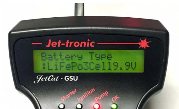
After the battery type has been correctly set, navigate to the parameter “Battery Size (mAh)” and set to the capacity of the engine battery. Per default “LiFePo3Cell 9.9V” with 2100mAh are supplied with the engine.
