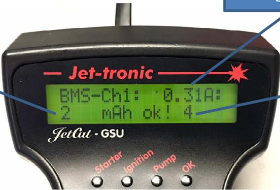
Last capacity charged into receiver battery #2 in mAh. In this example 1mAh had been charged last time.
