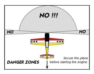
Make sure that the plane is secured properly when you start the engine. Have at least 2 helpers hold your plane from the tail end, or from behind the wing tips, before you start the engine. Make sure that all spectators are behind, or far in front, of the aircraft when running up the engine.
