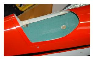
It is important to start the canopy glass installation with the frame mounted to the fuselage, with a piece of tape holding the rear frame/loop firm to guarantee a consistent gap to the fuselage rear deck. It is also easier to complete this stage before the motor dome is bolted in position, as it allows you to reach inside the fuselage to help position the glass during gluing.
