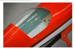
tacking on the glass edge, working in sections and replacing the frame after every few applications, checking for distortion, as you go. When you are happy you can either run around the edge with Hysol or ZAP 560 canopy glue to permanently fix the glass in place.
