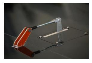
the servo screws supplied with your choice of servo. The screws are  $(2.9 \times 16)$ . The servo hatch is mounted to the wing with four  $2.9 \times 13$  sheet metal screws. Add tape to the drill bit to stop any chance of breaking through to the wings top skin when drilling the four servo hatch mounting holes.
