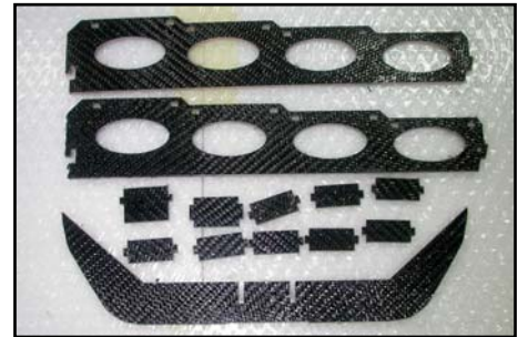
(above) The milled carbon/balsa parts for the rudder tray, and the end support bulkhead.
