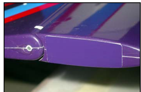
(above) Servo access hole in stab tip is covered with pre-painted fibreglass sheet included in the kit.
