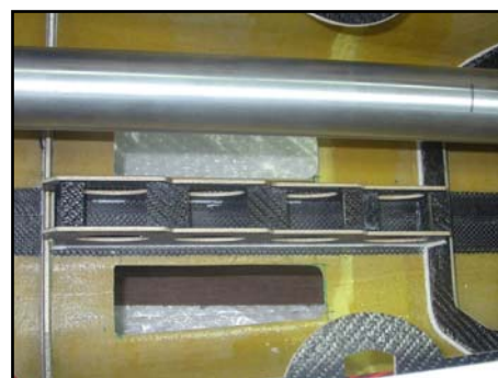
(above) Air exit slots either side of the rudder tray. Size 150 x 50mm. (below) Simple 3mm composite balsa baffle plate glued into the lower cowl for the DA-150.
