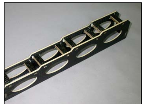
(below) The completed rudder tray is light and very stiff.
