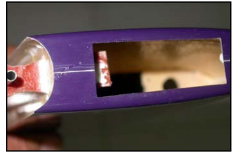
(above) Cut off inner end of outer phenolic hinge post if needed.
