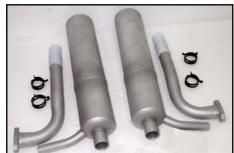
(above) We highly recommend the MTW canisters, headers and teflon connectors, which C-ARF can supply as an option.
