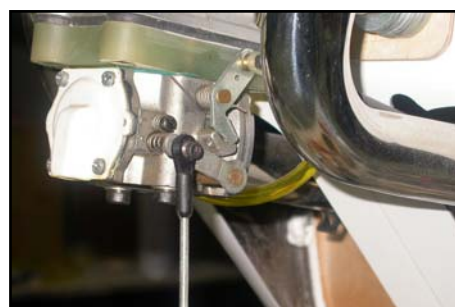
(below) A choke rod was made from M3 all-thread and a ball-link.
