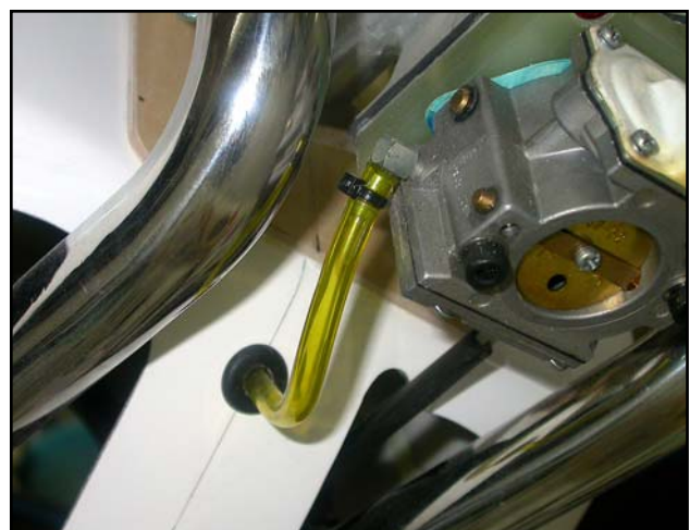
(above) Use a rubber grommet where the fuel tube passes through the firewall, and a cable tie to make sure it cannot come off the carb.
