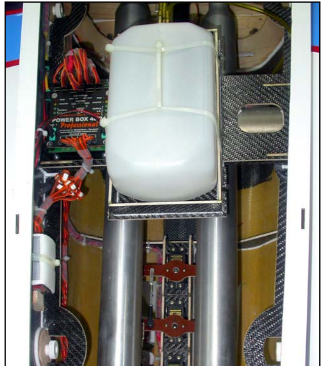
(above) General view of the R/C installation, with Powerbox on the fuel tank base, and receiver fixed to side of fuselage behind it. Keep all the wiring and tubes firmly fixed so they cannot rub on any composite material, or touch the hot exhaust system.
