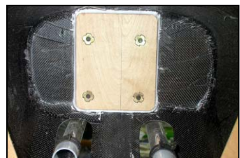
(above) M6 T-nuts on the inside of the plywood firewall. Secure with a little 30 min. epoxy.
