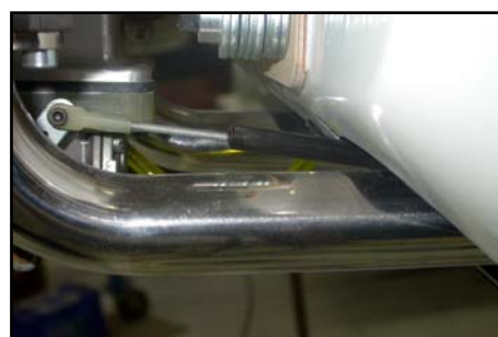
(below) A choke rod was made from M3 all-thread and a ball-link.
