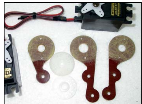
(below) The 3 phenolic servo arms, prepared before gluing and screwing into position.
