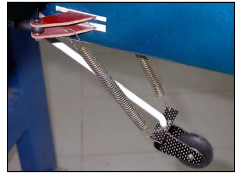
(above) Connect the steering arm to the rudder horns with springs for steering option if required. SuperXtra shown here.
