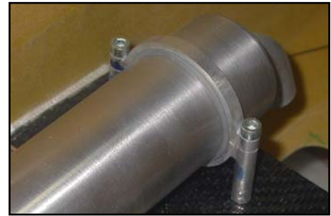
(above) Pipes are isolated from vibration with the silicone sleeves provided, under the clamps.
