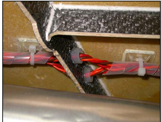
(above & below) It is very important to protect all tubes & wires where they pass thru' fibreglass or carbon parts, or near to composite milled parts, where they could be damaged due to vibrations. Use grommets or split silicone tube around the edges of holes in composite material, and plastic spiral-wrap.
