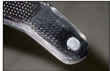
(above) The moulded dimple in the bottom of the carbon legs. Drill a central hole of 6mm diameter.
