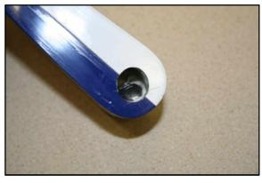
The stab tube is already complete and ready for you to use, no more needs to be done other than fit the tube to the stabs. The retention bolts have been pre fitted for you, and only requires you to fit the stabs to the fuselage. The stab tube may already be marked with L and R, to help you distinguish the correct orientation. If not, don't stress, it can only go one of two ways!
