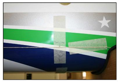
Place some masking tape on the fuselage roughly where your mark will be. With the straightedge on the canopy seat mark a line using the measurement you just established. Now that you have the servo arm position marked on the outside of the fuselage, you can use a string line to mark the horizontal cable line.
