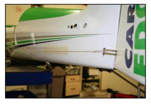
You can double check the exit measurement by running the string along the bottom of the fuselage. Flip the model upside down, and directly underneath the servo draw the servo arm measurements onto so masking tape. Remember this measurement is dependent on which servo arms you use.
