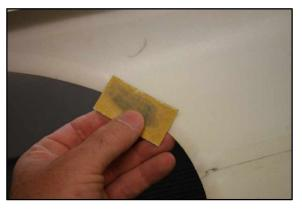
It's important that you fit the canopy while the canopy frame is attached to the fuselage, this will keep the frame properly aligned and not twisted. Masking tape is used to hold the canopy in position prior to gluing. It may pay to have another pair of hands available to assist you here. Perhaps you can bribe your best buddy with a beer, or two (after their assistance)!
