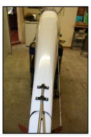
When you are satisfied that the cable exit slot is positioned correctly, make a cut with your Dremel and cut off wheel. The cut off wheel will cut the fuselage material with ease, so keep the tool steady.
